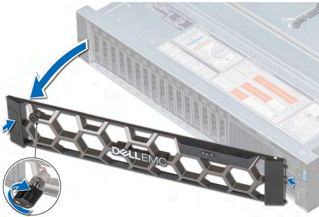
Figure 3 Removing the front bezel
