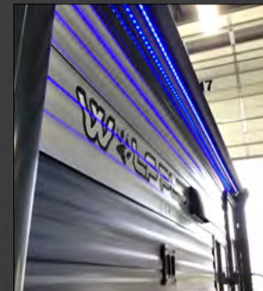
Exterior LED Light Strip at Awning
