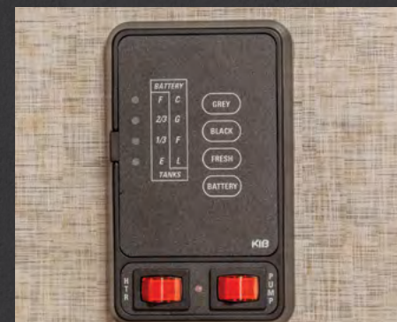
Monitor Panel for Tanks and Battery Levels
