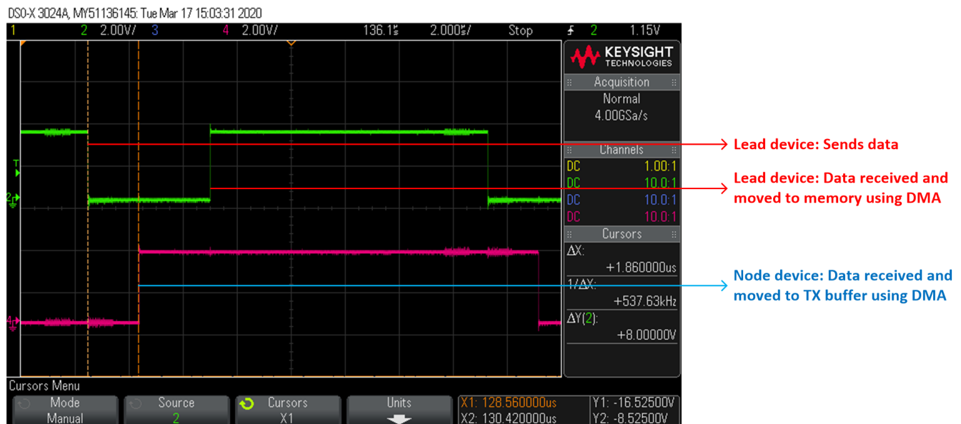
Figure 5-4. FSI Communication Using DMA Control
