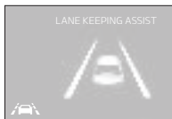
When the front-view camera does not detect the lane traveling in, the lanes are not illuminated
