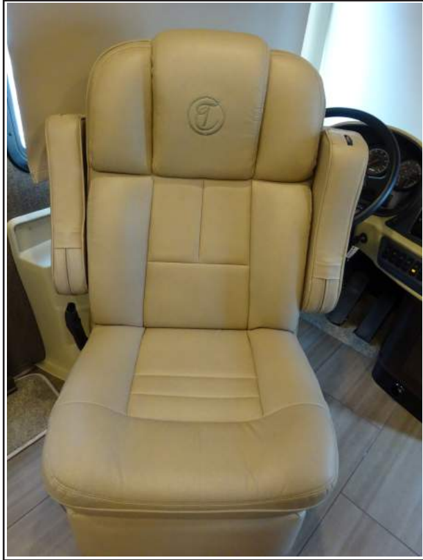
Figure 7-5: Both the driver and passenger chairs swivel to face the living area of the coach
