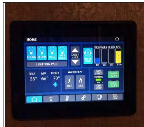
Figure 13-5: Water pump switch
