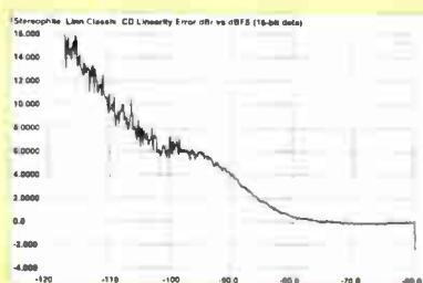
Fig.4 Linn Classik, left-channel departure from linearity, 16-bit data (2dB/vertical div).
