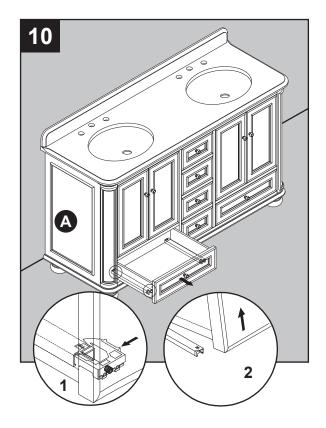
11. To re-install drawers into vanity (A). Please fully extend metal glide tracks, gently lower and slide drawer box into rear glide catch, then, lower drawer box down to completely rest on extended glides, push plastic levers to lock the drawer box in place.
