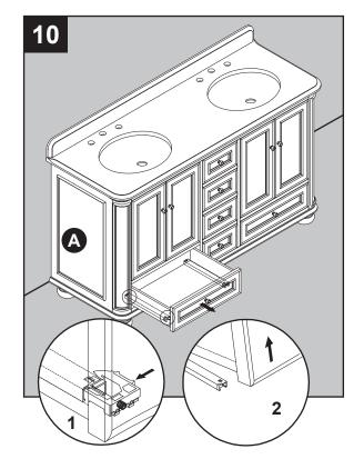
11. To re-install drawers into vanity (A). Please fully extend metal glide tracks, gently lower and slide drawer box into rear glide catch, then, lower drawer box down to completely rest on extended glides, push plastic levers to lock the drawer box in place. Repeat for remaining drawers.
