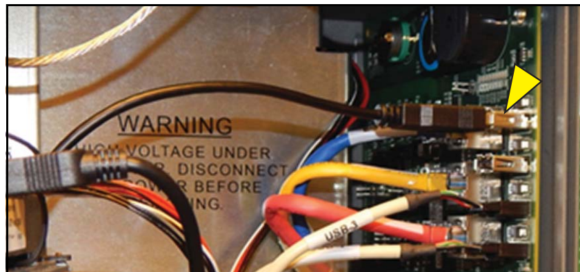
Figure 20. Connect Optional Printer USB Cable
