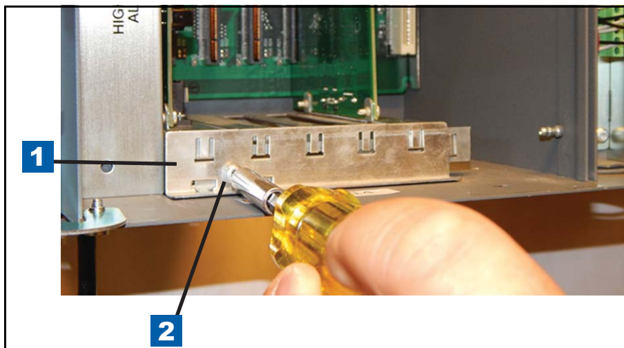
Figure 10. Removing Comm Module Clamp
