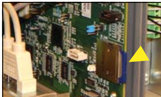
Figure 24. Locating SD Card On CPU Board
