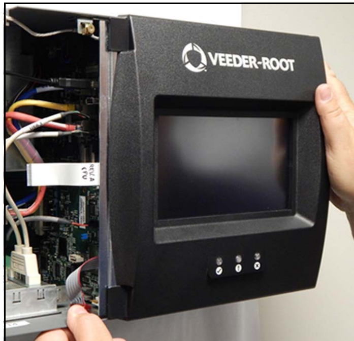
Figure 21. Install The New TLS-450PLUS Display Door
