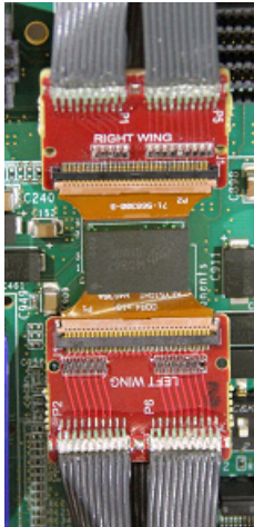
Figure 47 W4636A interposer attached to E5847A ZIF connectors
