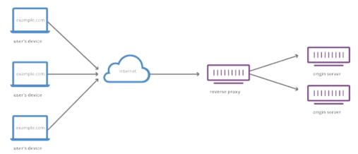
Before devices outside the OT network can access the Web Client, a reverse proxy must be configured on the DMZ server. AVEVA Identity Manager must be enabled for the reverse proxy to function. There are many providers of reverse proxy solutions. Refer to the relevant reverse proxy solution documentation, for instructions on setting up the reverse proxy solution in your infrastructure. For more information, see the InTouch HMI Application Management and Extension Guide.
