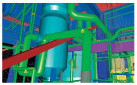
The automated Pipe Run feature lets users select points on connected, straight pipe sections, and the system automatically models a best fit pipe run with elbows in seconds.
