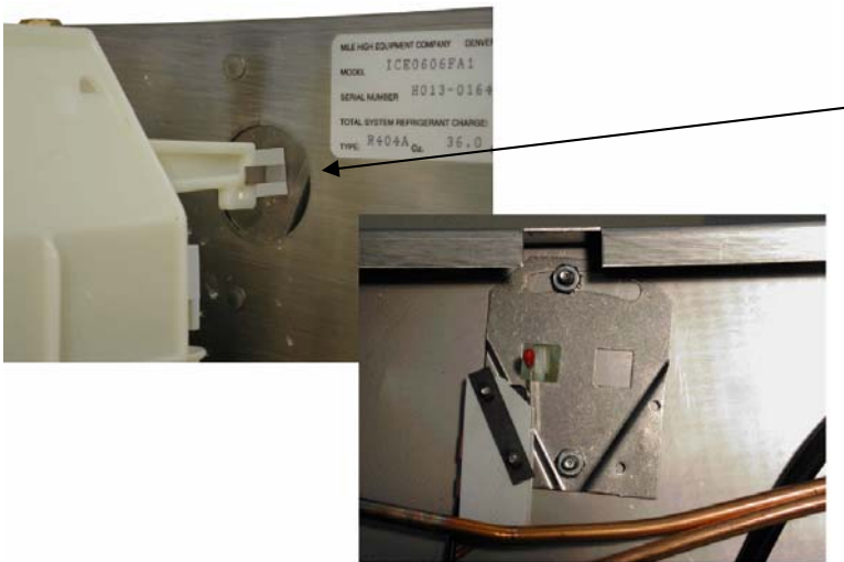
Proper position of wire bale switch actuator
