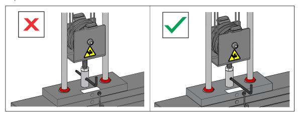
**3.** When proper thread engagement is reached, tighten jam nut to 20-25 FT-LBS (27.2 - 34.0 Nm) using a 24mm wrench.
