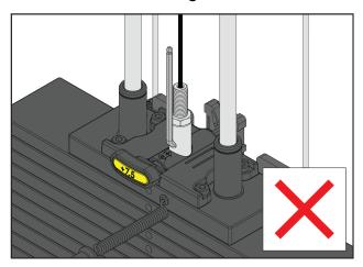
18. Select either the LBS or KG weight stack label. Remove backing from label and apply to weight stack.
