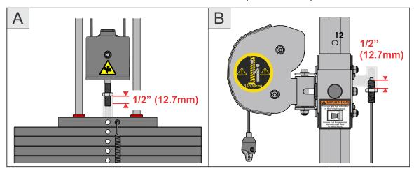
2. Certain models are now equipped with a bayonet portal to assist checking proper thread engagement. To do so, attempt to pass a 7mm Allen wrench through the portal, if it goes through, more threads are needed to meet the minimum requirement.
