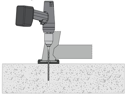
**4.** Insert fastener and tighten to 18 Foot-Pounds (24Nm) for 1/4" (6mm) anchor or 40 Foot-Pounds (54Nm) for 3/8" (8mm) anchor.
