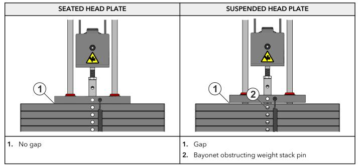
2. Ensure that the weight stack selector pin can fully engage into each weight plate.
