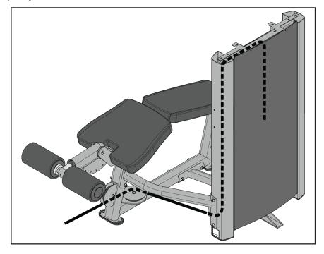
**21.** Install cable clip securing the cable to the cam.
