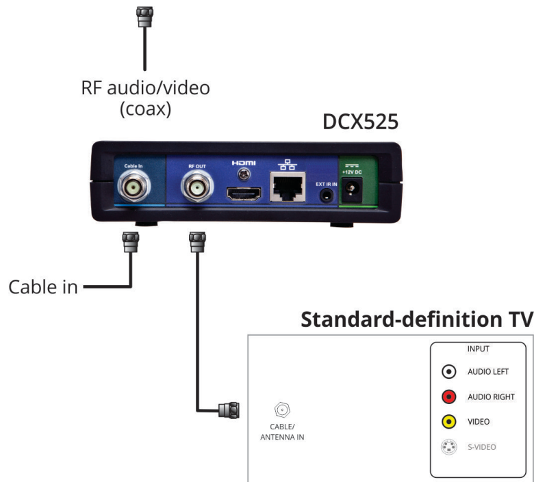
Figure 4: Connecting an SDTV — Single Connection for Video/Audio
