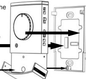
2. Secure the thermostat Power Module into the box with the mounting screws provided.
