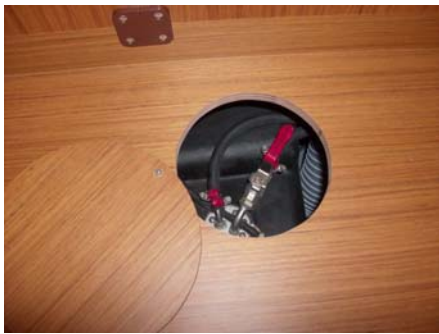
Valve - Sea water inlet valve for engine (Reference 1)
