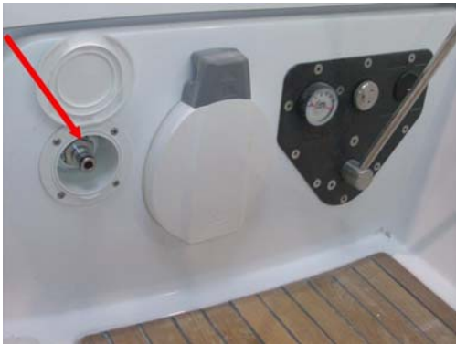
SOCKET - SHORE WATER Location
