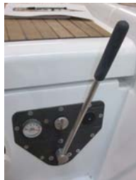
Backstay - Hydraulic (optional) Cable adjustment
