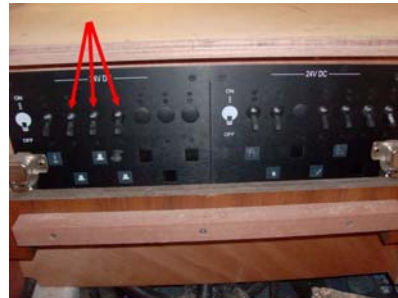
Circuit breakers Location: Starboard saloon Genoa sheet winches - 100A Spinnaker sheet winches - 60A Rigging winches - 60A
