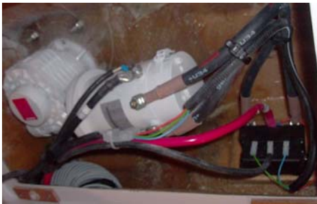
Genoa sheet winches Engine - 24V + Relay box Access: Deckhead - Cabins
