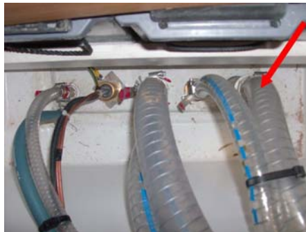
Valve - Sea water inlet valve for engine (Reference 1)
