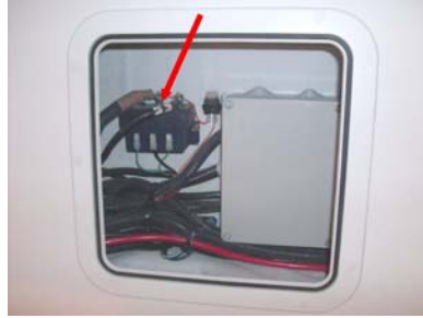
Circuit breakers Location: Starboard saloon Genoa sheet winches - 100A Spinnaker sheet winches - 60A Rigging winches - 60A
