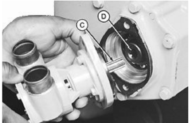
Install sea water pump. Splined shaft (C), Drive Gear Splined ID (D)
