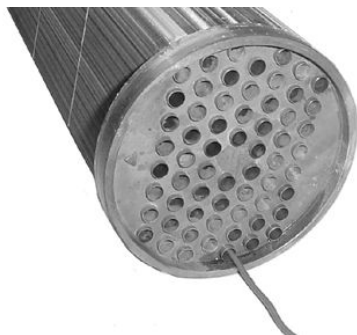
Aftercooler core cleaning
