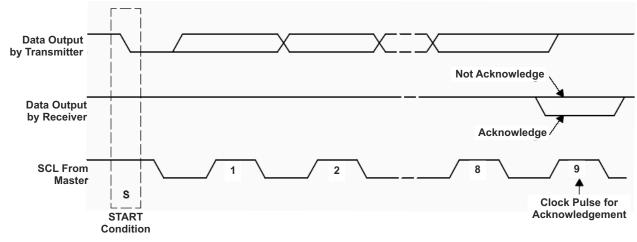
Figure 9-11. Acknowledge on the I<sup>2</sup>C Bus
