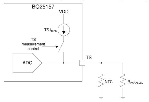
$R_{PARALLEL} = R_{NTC@25C}$
