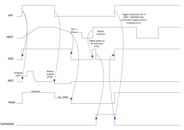
Figure 9-14. BQ25157 Wake-Up Upon Supply Insertion
