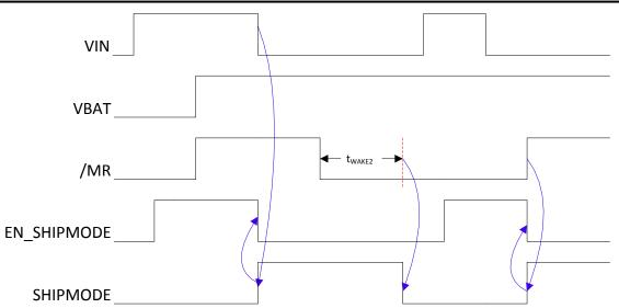
Figure 9-13. Ship Mode Entry Based On EN\_SHIPMODE bit
