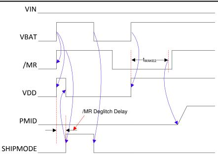
Figure 9-15. BQ25157 Wake-Up Upon Battery Insertion
