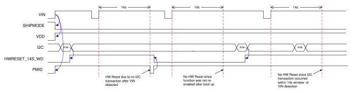
Figure 9-7. 14-Second Watchdog for HW Reset Behavior
