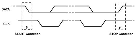
Figure 9-9. START and STOP Condition
