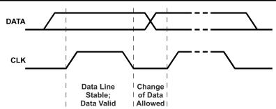
Figure 9-10. Bit Transfer on the Serial Interface
