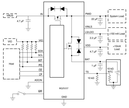
Figure 10-1. Typical Application Diagram
