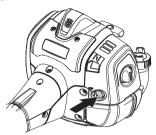
(2) Choke: Move choke control up to choke position.
