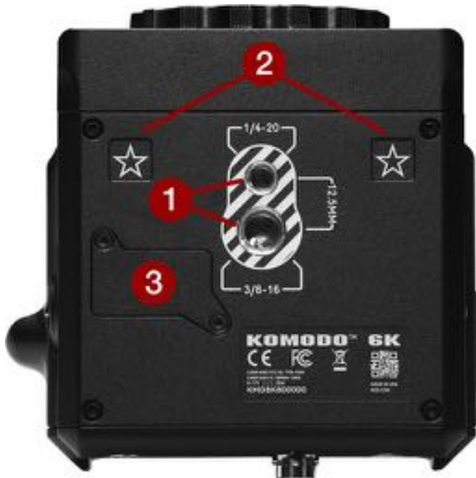
Figure: Camera Body Bottom Controls and Features
