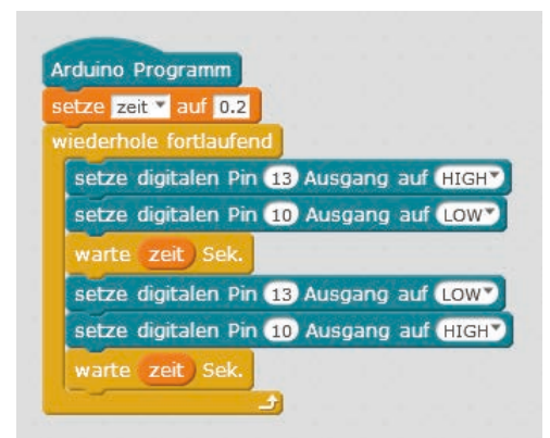
The program 03mb1ock lets two LEDs to flash alternately with adjustable speed.
