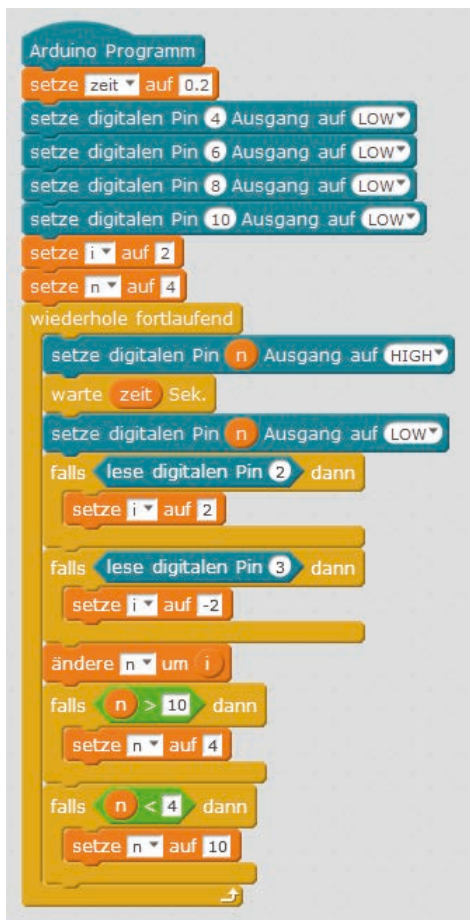
Direction switch of chaser light with two buttons.
