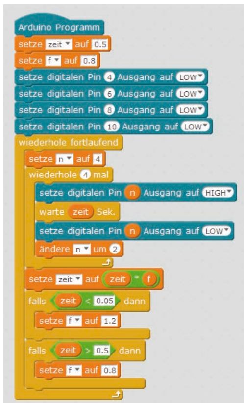
The 10mblock program lets the LEDs light up as a chaser with variable speed.
