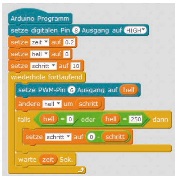
The program 08mb1ock dims an LED at the PWM output.
