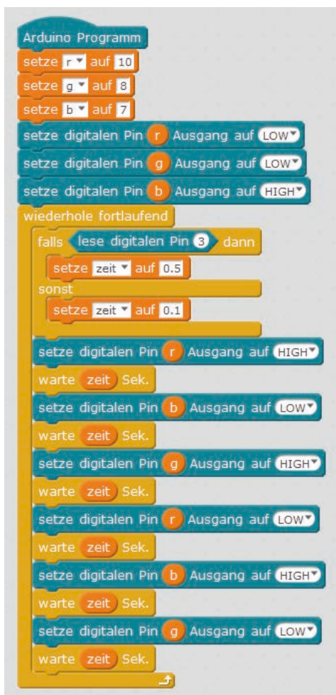
The 12mblock program switches an RGB LED and individual LEDs.
