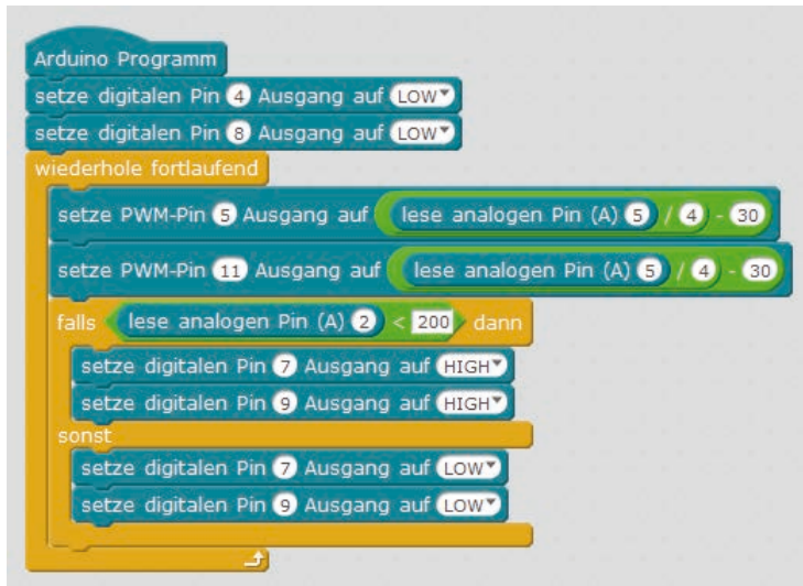
The 16mBlock program controls two RGB LEDs via a potentiometer and a sensor contact.
