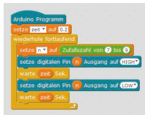
The program 07mblock01 lets three LEDs flash randomly.
