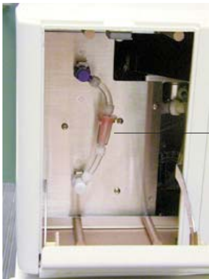
Fig. 3A. Sheath filter internal fluidics features.
