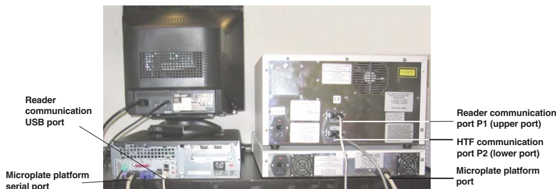
Fig. 12. Completed connections of computer and monitor to the Bio-Plex suspension array system.
