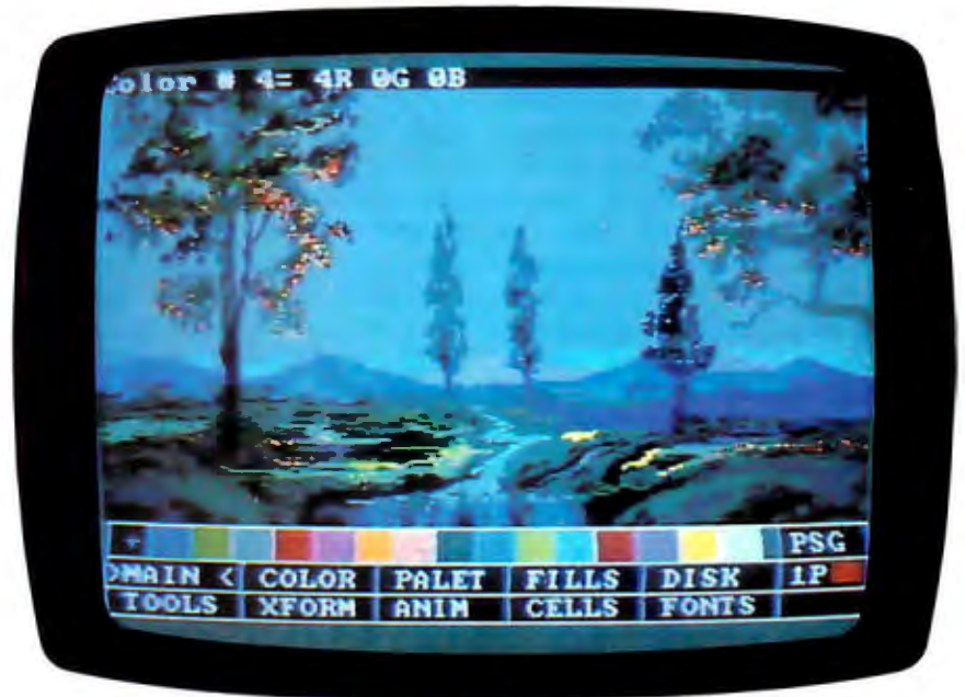
Photo 3: An example of graphics produced by the Mindset using Lumena software and an IBM PC-compatible RGB monitor. The photo shows the Lumena control panel. This display is overlaid on your drawing when the cursor is moved through the bottom of the screen. Moving the cursor out of the control panel restores the screen to its original condition.
