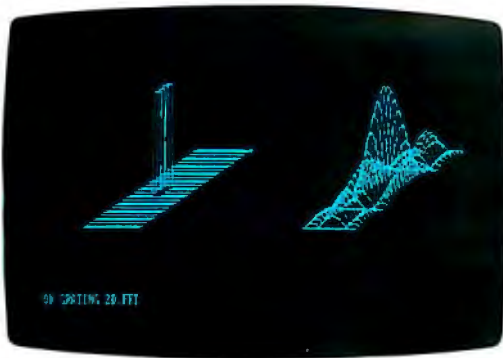
ASYST multiple windows permit side-by-side comparisons. The two-dimensional FFT routine, shown, is one of the many built-in functions.
