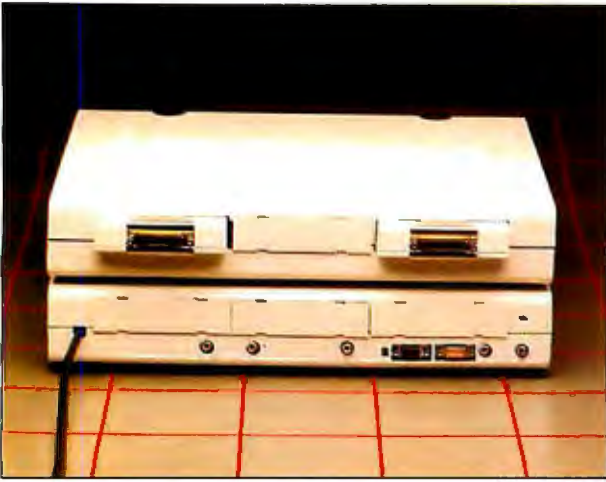
The rear panel of the Mindset system unit and expansion unit. Note the three slots on each for I/O modules.
