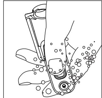
3 Use the toothbrush to scrub off any dirt or foreign matter from the niches of the top catch and thumb screw.
