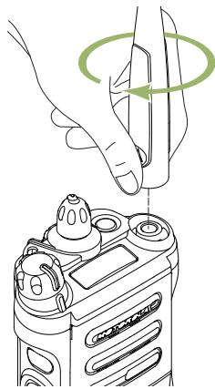
3 To remove the antenna, turn the antenna counterclockwise.
