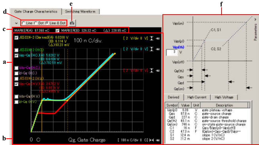
Figure 4-26 Gate Charge Characteristics
