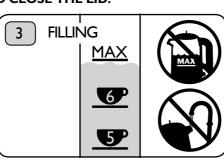
Fill the kettle through the lid opening. Use at least one cup of water (250ml). The water level must stay below the 'max' mark. Save energy, only boil what you require. Keep kettle upright and level at all times when filling. Do not tilt kettle backwards. **DO NOT OVERFILL OR**
