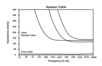
Dynaudio Ocos has succeeded in producing a loudspeaker cable that fulfills the conditions for optimum matching and signal transmission. All prior experience – that thicker cables offer improved performance – coincides with the behavior of characteristic impedance.
