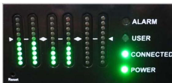
Stereo connection with PPMs 1-4 displaying input and return audio
