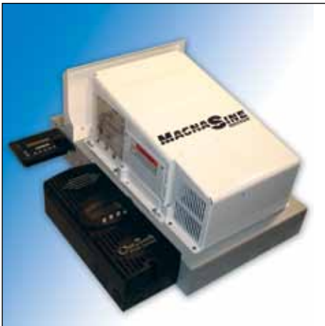
SunWize Power Center Assembly with MidNite E-Panel, Magnum MS inverter and charge controller (shown without mounting brackets). These power centers combine the disconnects, overcurrent protection devices & controls into an easy-to-install and operate panel. All include 50' MS Remote Control (shown top left).
