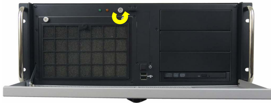
Figure 27: Loosening knurled screw on the rear side
