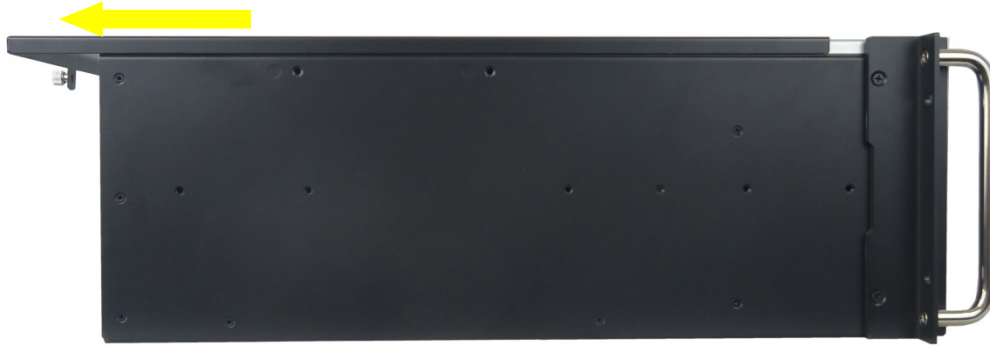
Figure 29: Removing the cover
