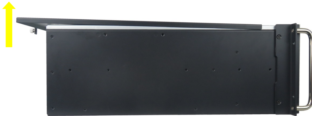
Figure 29: Removing the cover
