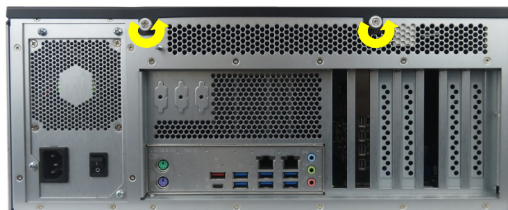
Figure 27: Loosening knurled screw on the rear side
