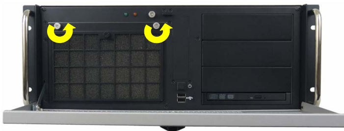
Figure 44: Fan compartment (without fan assembly)
