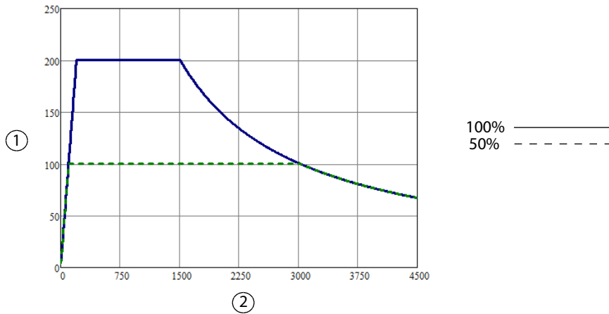
Output power versus resistance for BLEND power
