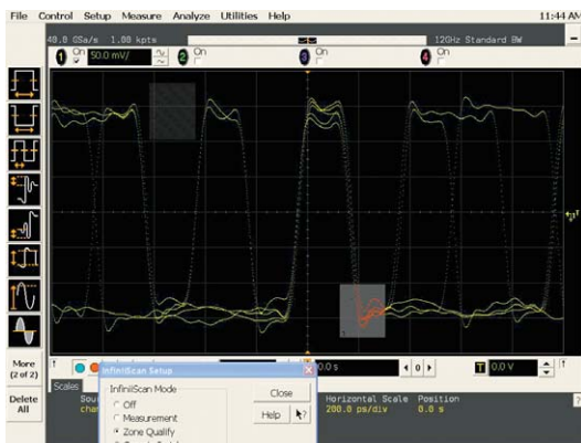
The "true" ease of use. Just draw boxes and the scope will trigger. The industry's only software event finder, "InfiniScan Event Identification Tool" will provide the next level of ease-of-use for the scope triggering system.
