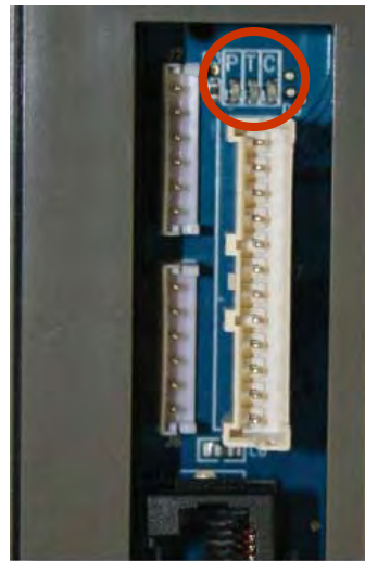
T7 EPP's three LEDs are P, T, C (left to right)
