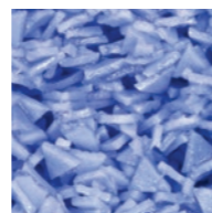
3M Precision-Shaped Grain (Sintered corundum)
