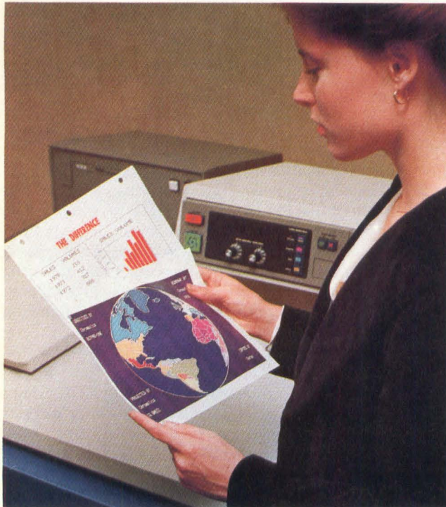
Figure 2: The 6500 color printer from Xerox combines laser scanning and xerography to produce 3 pages/min with 100 dot/in resolution.
