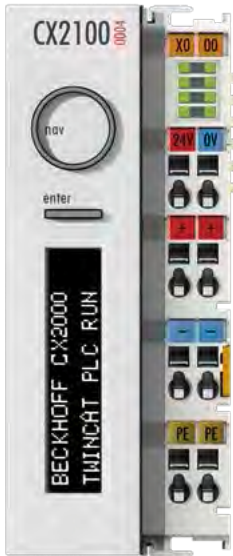
Power supply unit with E-bus/K-bus interface
