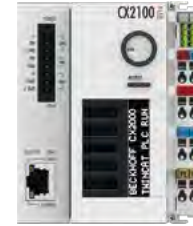
Power supply unit with integrated Smart Battery charger and E-bus/K-bus interface
