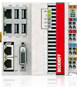
CX5020 with optional PROFINET interfaces
