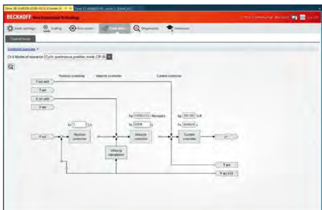
Direct fine-tuning of the drive during commissioning
