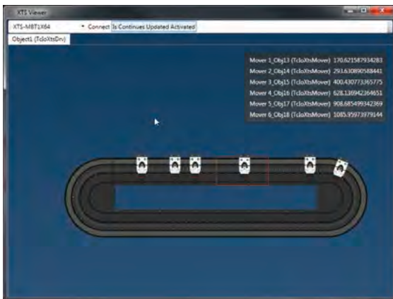
The XTS viewer renders an intuitive online 2D representation of the movers in motion and can be used as a diagnostics and simulation tool.
