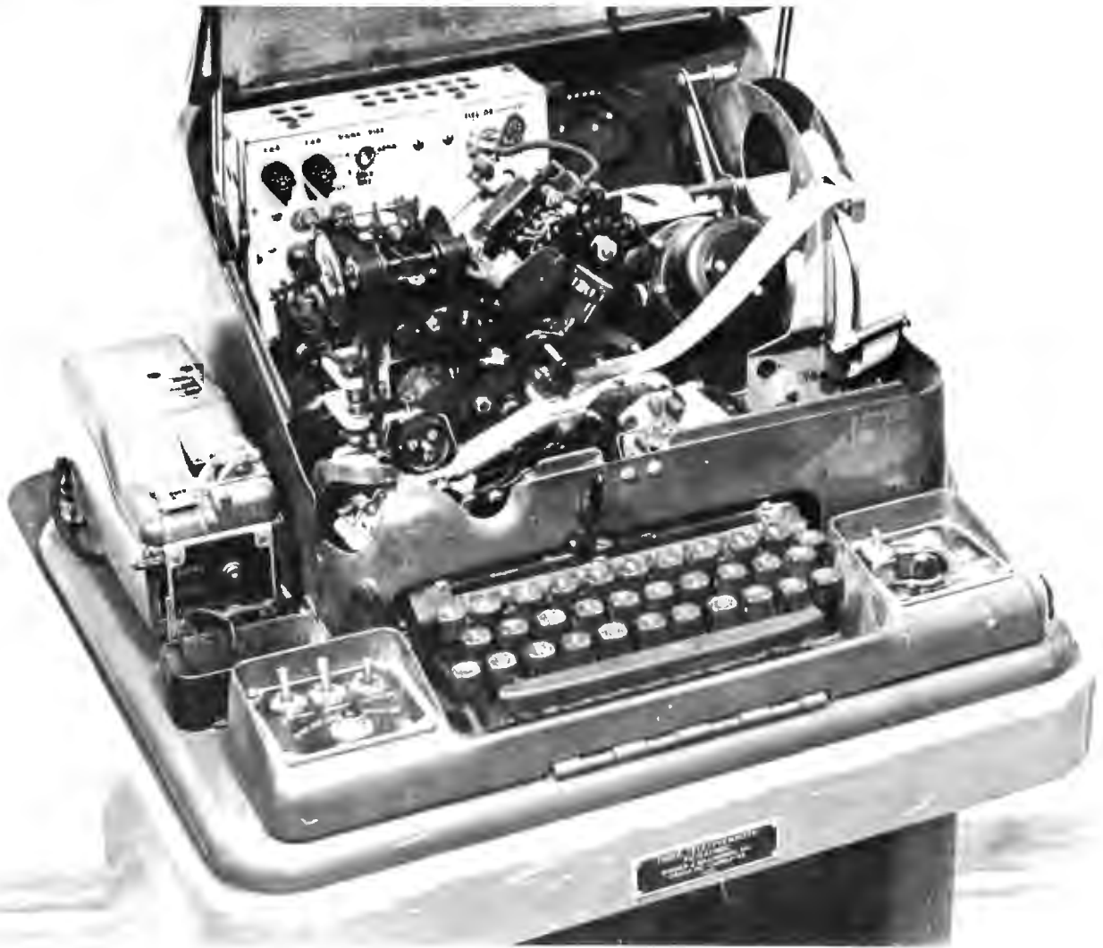
Photo 5: A view with cover lifted of the author's Kleinschmidt Model TT-76A (military nomenclature). This machine is a paper tape punch and reader only, which actually types characters on the tape. Like the Kleinschmidt in photo 4, this unit contains a loop power supply.
