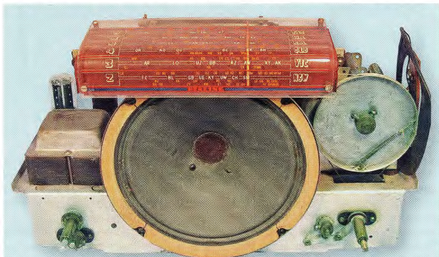
This front view of a 502E chassis shows the unusual curved dial-face and the mechanical linkages used for the on/off switch (right) and the tone control (left).
