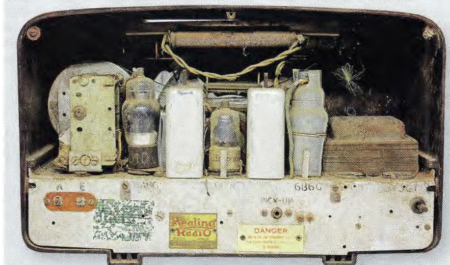
The author's L502E receiver prior to restoration. It was covered in dust, had missing knobs and valves, and came with spider webs and a wasp nest.
