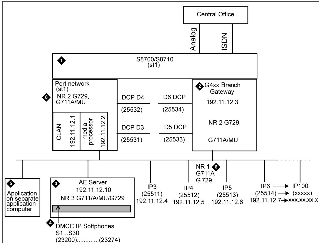
1. Communication Manager - Supported media server with a CLAN circuit card and a media processor circuit card
