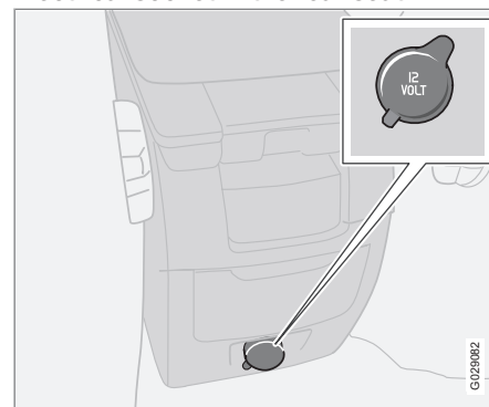
Electrical socket in the rear seat.
