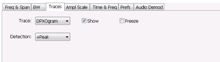
Traces tab – DPXogram trace (RSA6100B and RSA5100A with Option 200)
