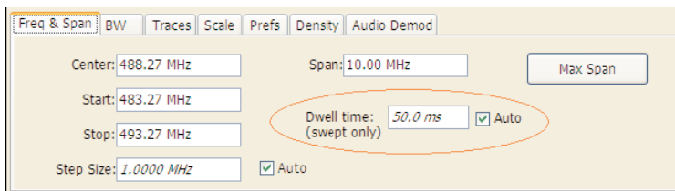
Figure 15. During swept DPX operation, the Dwell time control adjusts the observation time of each frequency segment used to construct the composite DPX display.
