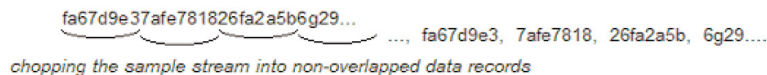
Figure 4b. Samples are segmented into data records for FFT processing based on the selected resolution bandwidth.
