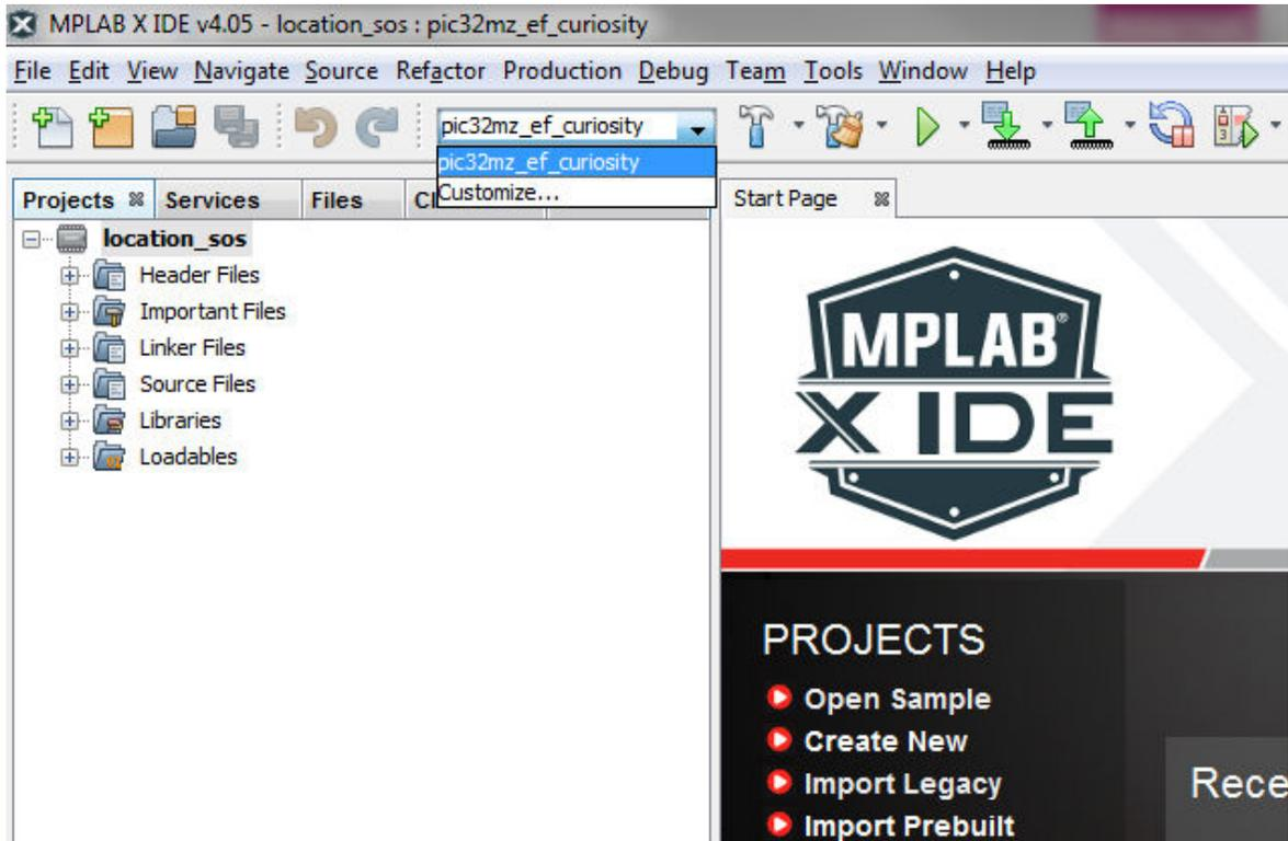
4. The *pic32mz\_ef\_curiosity* configuration arranges MPLAB X IDE to build and run the demonstration application on the PIC32MZ EF Curiosity Development Board, with the PIC32MZ2048EFM100 microcontroller.
