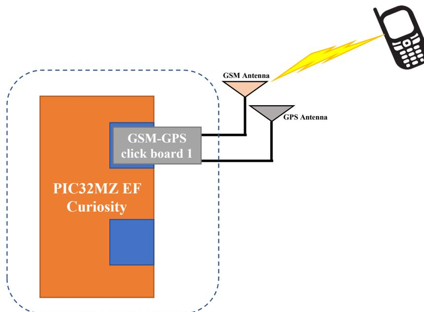
On power up, the application interacts with the GPS module on the GSM-GPS click board over the UART interface to perform the acquisition and tracking of GPS satellites. It registers the event callbacks for location tracking of the GPS receiver.
