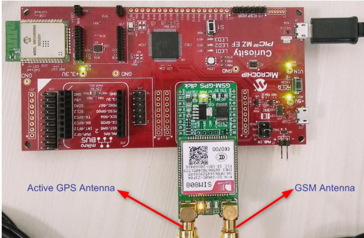
3. Power the PIC32MZ EF Curiosity Development Board from a host PC through a Type-A male to Micro-B USB cable connected to Micro-B port (J3). The cable is not included with the kit. Ensure that a jumper is placed in J8 header (between pins 4 & 3) to select the supply from the debug USB connector.
