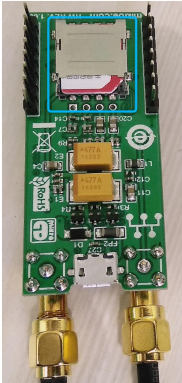
2. Mount the GSM-GPS click board on the mikroBUS socket J5, and connect the GPS and GSM antennas.
