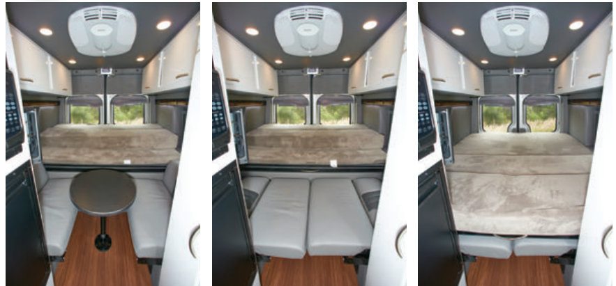
To convert the rear area for sleeping, the rear jackknife seats fold down, the platform moves into place and the cushions are placed on top. Side window pods offer additional sleep-position options.
