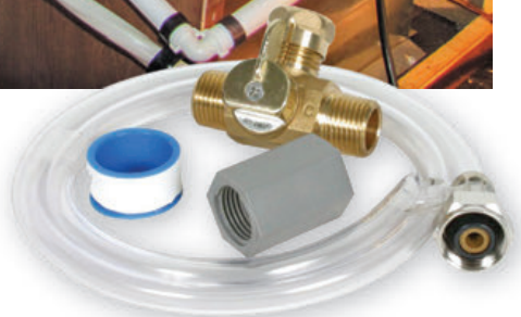
[6] When there is no winterizing kit, the hose is disconnected from the inlet side of the pump's inline filter, and a 3-foot suction hose with a 1/2-inch NPT female PEX fitting clamped on the end is attached. You can get these parts at most home centers. An alternative would be to install a pump converter winterizing kit made by Camco.
