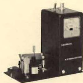
C2 Test Head with VU Meter and Pre-Amplifier
