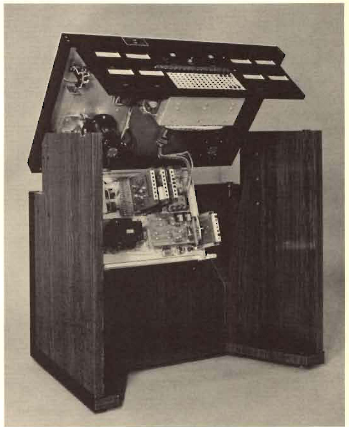
Model 1210 tilt-up console cabinet.
