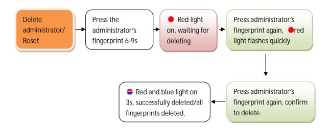
Notes: It's warning signal that factory settings will be restored soon when the red light flashes quickly, wait for 10 seconds to automatically exit the delete mode if you don't want.
