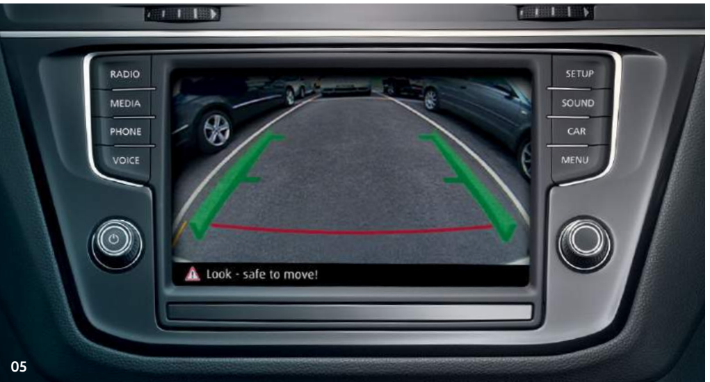
05 The rear-view camera , which forms part of the Park Assist and Trailer Assist options, is integrated behind the Volkswagen badge on the rear tailgate, displays the area behind your vehicle on the screen of the vehicle's audio system, helping you to manoeuvre into tight spaces quickly and easily. Auxiliary lines help you navigate safely into parking spaces, and thanks to the high resolution display, even small obstacles such as kerbs are visible. Optional on SE models and above.
