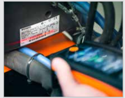
ArcValidator RC records all individual validation process data for later transfer to the PC software.
