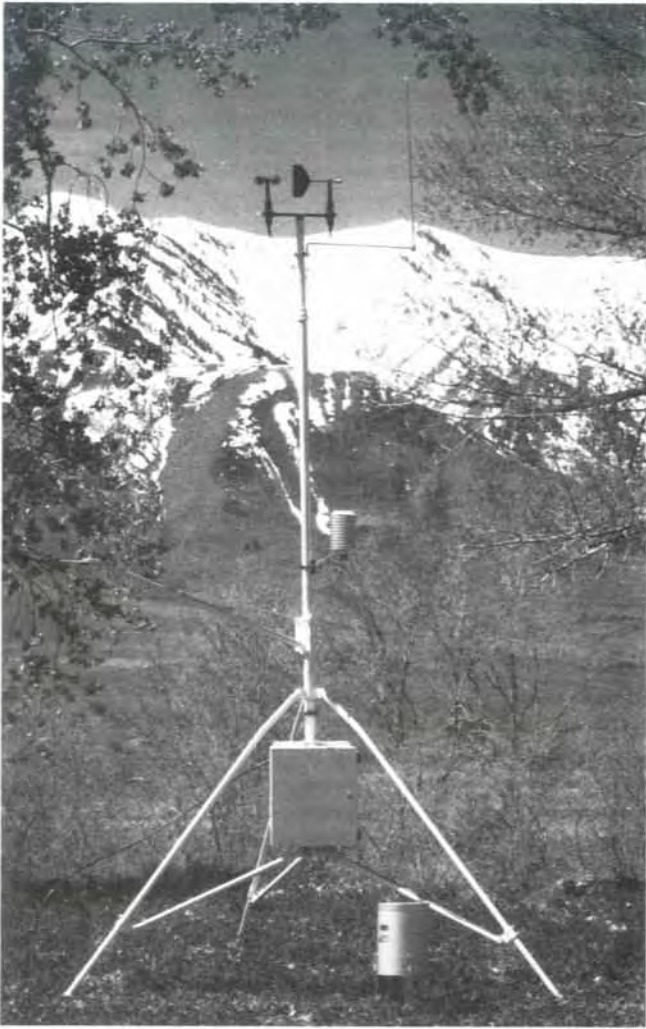
Figure 44.3 —Easy Logger recording system (Omnidata International, Inc.), with Wind Sentry (R.M. Young Co.) anemometer and wind vane, tipping bucket rain gauge (Sierra-Misco, Inc., model 2501), Gill multiplate radiation shield (R.M. Young Co.) housing temperature and relative humidity probe (Phys-Chemical Research Corp.), and pyranometer (Li-Cor). (Photo courtesy of Omnidata International, Inc.)
