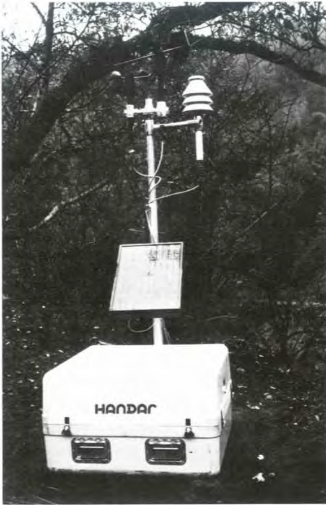
Figure 38.3—A “very portable” RAWS (“Micro-RAWS”). (Photo courtesy of Handar.)
