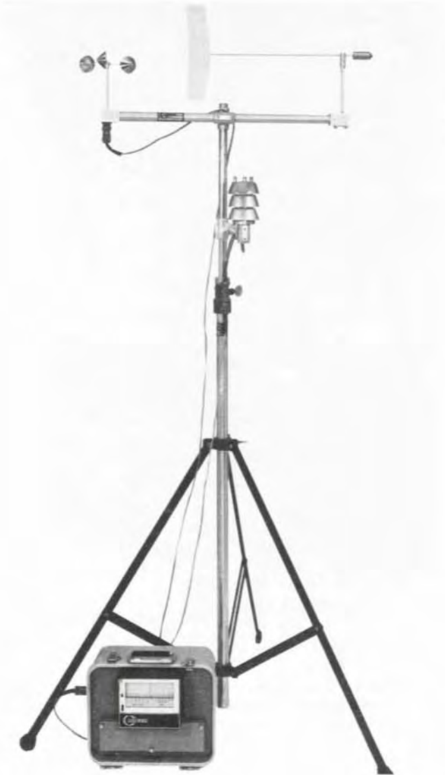
Figure 44.2 —Climatronics Electronic Weather Station (EWS), with on-site multiplex strip chart recorder. (Photo courtesy of Climatronics Corp.)
