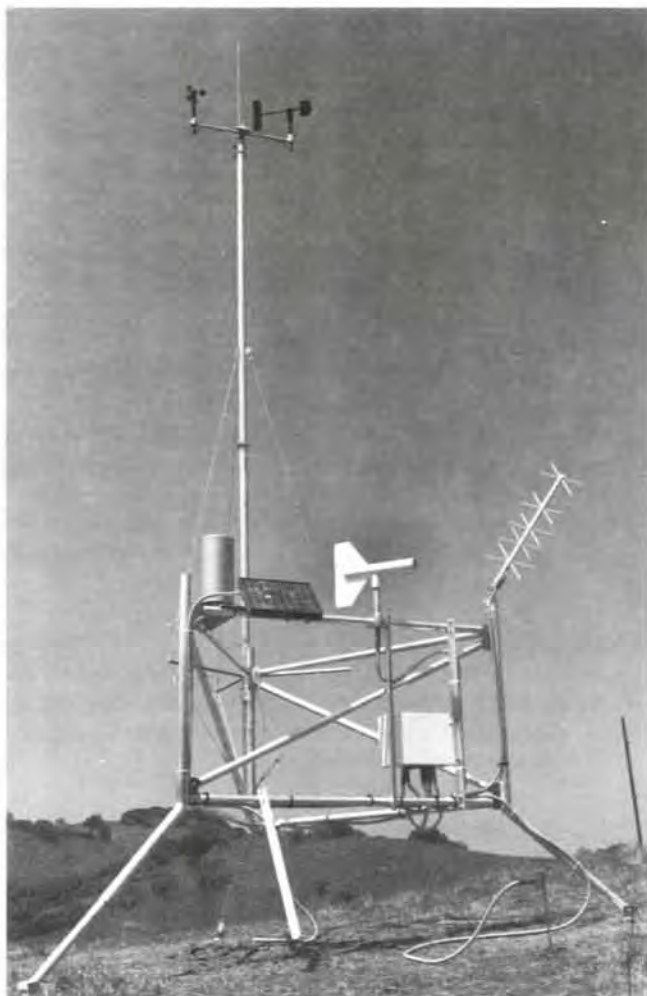
Figure 38.1 —View of standard Remote Automatic Weather Station (RAWS), showing tripod tower with sensors, solar panel, electronics enclosure (data collection platform), and GOES satellite antenna. (Photo courtesy of Handar.)
