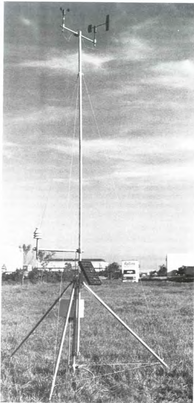
Figure 38.2—A portable RAWS, without satellite antenna. (Photo courtesy of Handar.)
