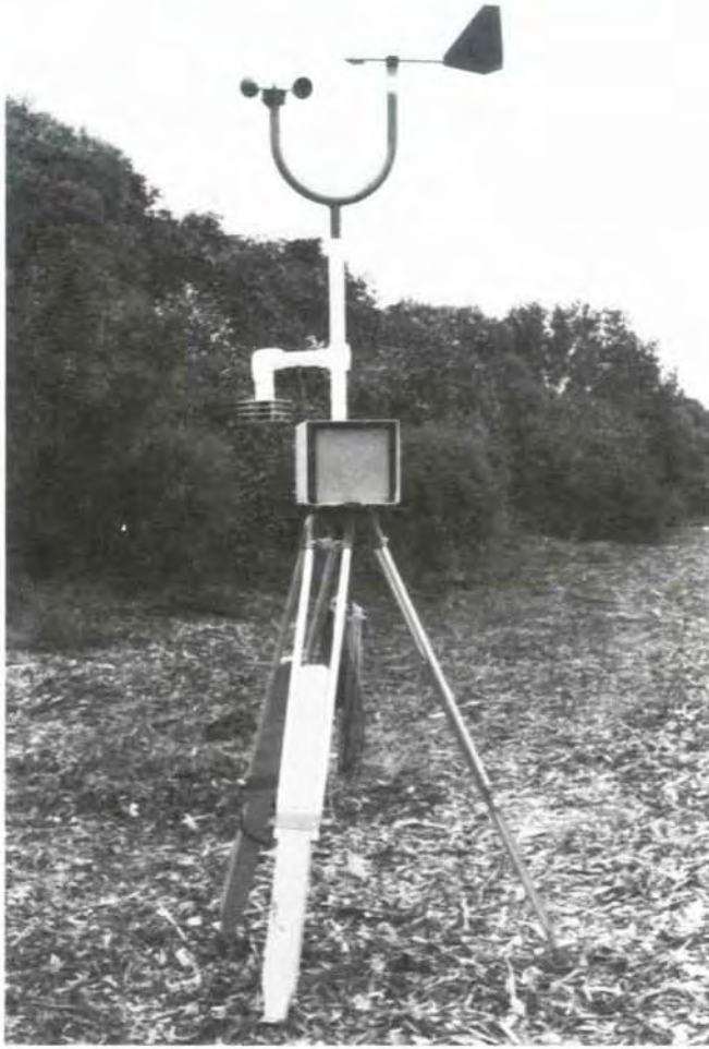
Figure 44.5 —CompuLogger (Sierra-Misco, model 6500) data collection system, with infrared transmitter and basic sensors; temperature/relative humidity probe is mounted in flat-plate radiation shield. (Photo courtesy of Sierra-Misco, Inc.)
