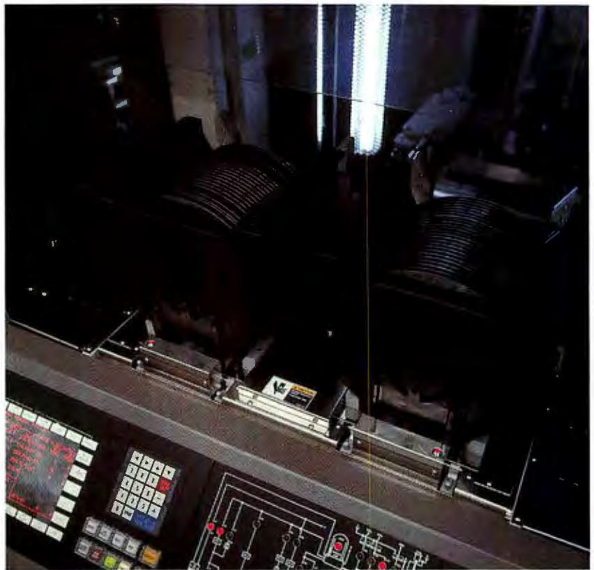
An implantation unit uses an electric field to embed trace elements in silicon and change its electrical properties.
