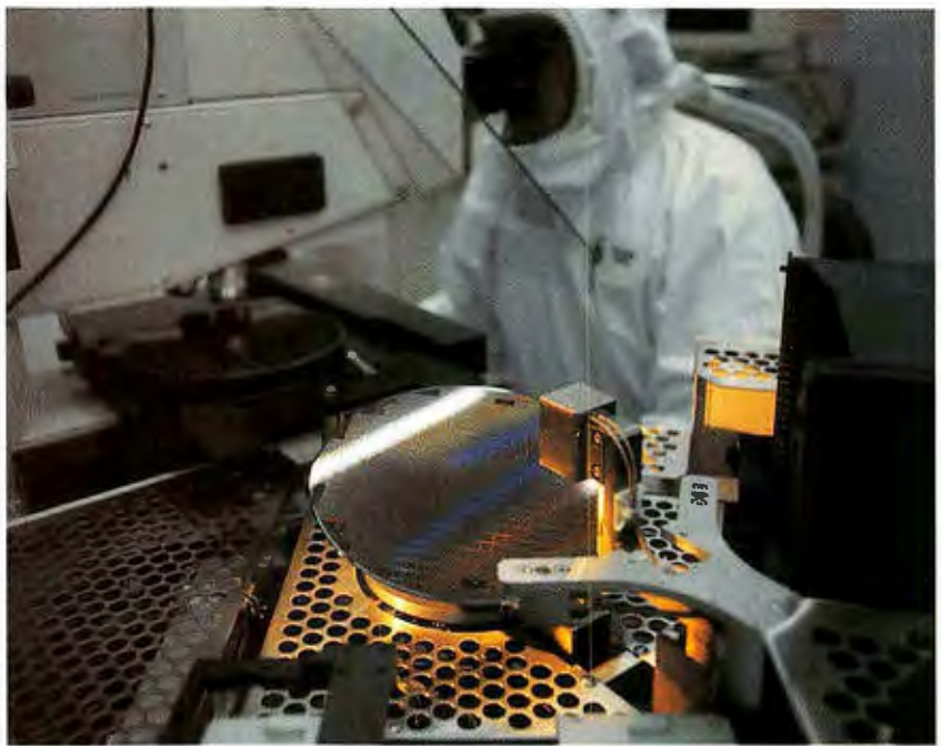
Rigorous testing, using machines and human inspection, finds defects in about 10 percent of the processors produced at Fab 6.
