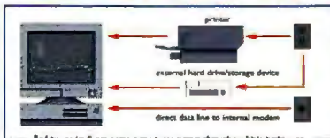
Bad power (red) can enter a computer system through multiple paths – eg. printer, data and phone/cable lines – even if computer AC is protected.
